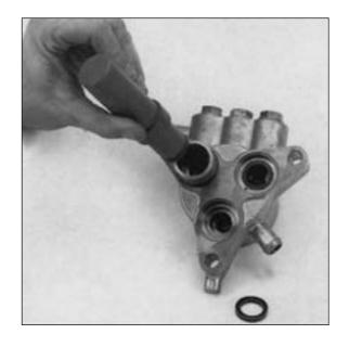
4.3 Leakage between the cylinder head and the pump housing
