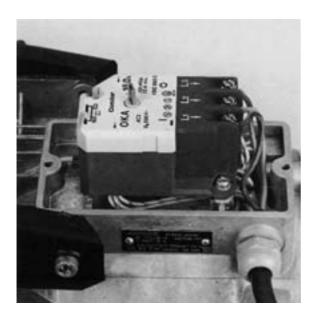
Phases L1, L2 and L3 are connected to the motor by way of the cleaner's motor protective switch Q1 (with integral thermal overload protection).
