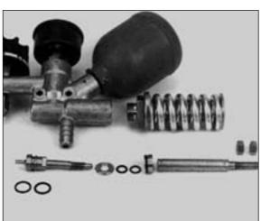
**Caution:** It is important for O-rings and support rings to be greased with silicon grease before mounting and that they be inserted correctly.
