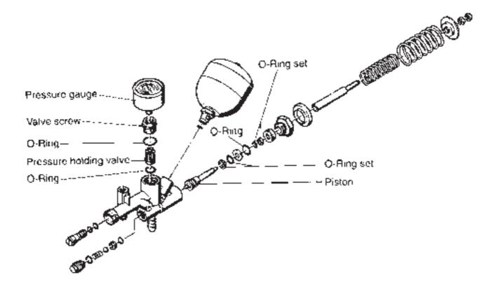
Dismantle the relief valve completly.
