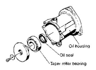
6.2 Ball bearing and seal defective
