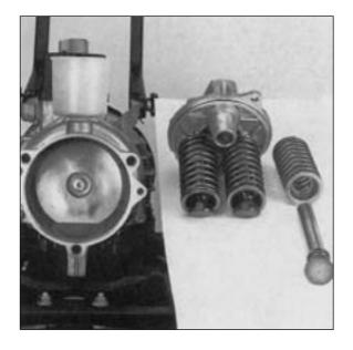
Insert the pistons and springs in the housing
