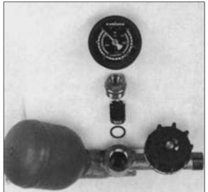
Replace the O-ring set of the piston and the O-ring set of the bushing, greasing the new parts with silicon grease before fitting.
